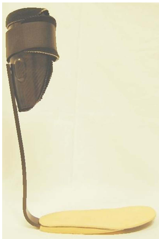
Figure 2 The experimental AFO. The stiffness of the AFO can be varied by exchanging the dorsal leaf spring. In total, five different springs (ranging in stiffness from very flexible to very stiff) will be assessed. AFO, ankle-foot-orthosis.
